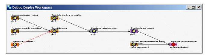
6 Constructs another suspected cause "Upstream and downstream limits are not large enough" on symcure-application-1 of "Incomplete specific fault model" and all its suspected causes up to the root causes. This figure shows the results after clicking Next seven times.
