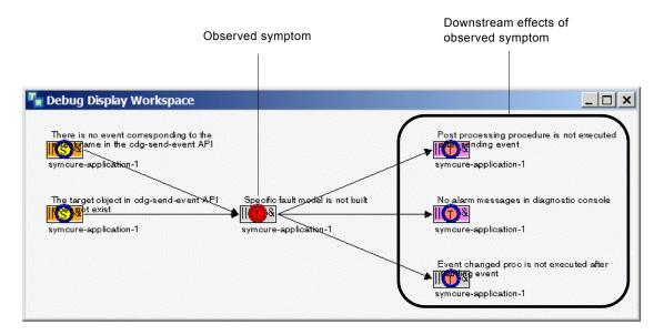
**4** "Specific fault model is not built" on **symcure-application-1** is observed to be false. The diagnosis manager propagates event value upstream. Both upstream root causes are inferred to be false.
