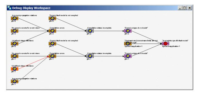
7 After constructing all upstream causes up to the root causes, constructs the two downstream effects of "Incomplete specific fault model". This figure shows the results after clicking Next twice.
