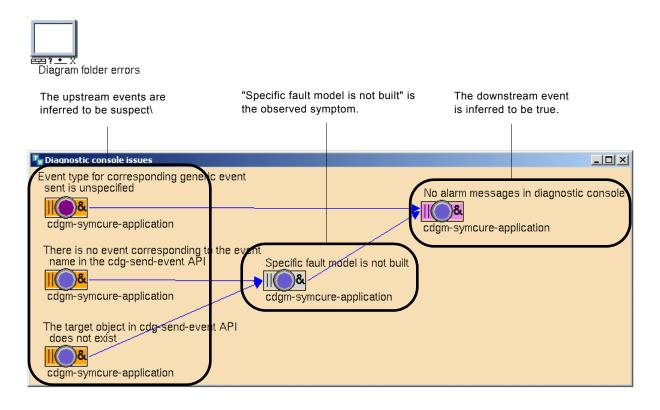
Here is the "Procedure execution" generic fault model, which defines generic event views for the "Specific fault model is not built" generic event, which defines additional downstream effects of the "Specific fault model is not built" generic event.
