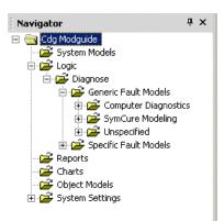
The demo provides two generic fault models, one for computer diagnostics and the other for SymCure application diagnostics. The generic fault models describe causal relationships between events and external actions that the model can run during diagnosis. SymCure creates specific fault models for domain objects at run time to diagnose faults.
