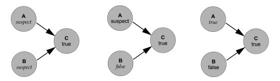
In this example, initially C becomes true, which causes A and B to be suspect. When B changes from suspect to false, A is the last remaining suspect event. Thus, for C to be true, A must be true. Hence, instead of making C suspect according to the OR logic rule above, SymCure sets A to be true.
