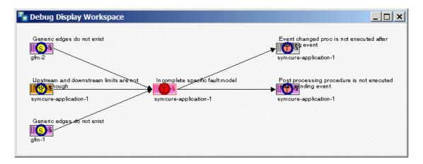
Note that the current event is still "Incomplete specific fault model". This is crucial to understanding parallel mode. As explained earlier, in parallel mode, the debugger alternates between navigating to a neighboring event and showing the neighbors of the current event, in parallel.
