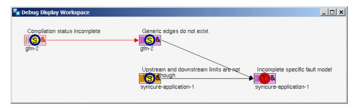
5 Constructs all the upstream causes of "Generic edges do not exist" on gfm-2. Note that in sequential mode, SymCure builds all upstream causes of each upstream cause until it gets to the root causes before it goes on to the next upstream cause. This figure shows the results after clicking Next five times.
