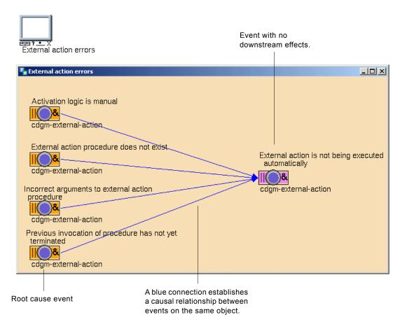
Here is the "Activation logic is manual" event and its properties dialog, which applies to the cdgm-external-action class:
