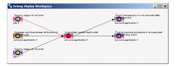
Note that parallel mode requires a number of extra steps to get to "Generic edges do not exit" on gfm-1 as the Current Event. This is because of the extra EXPAND-EVENT step for each event. While parallel mode overcomes the disadvantage of sequential mode by displaying all causes and effects of an event in a single step, it
