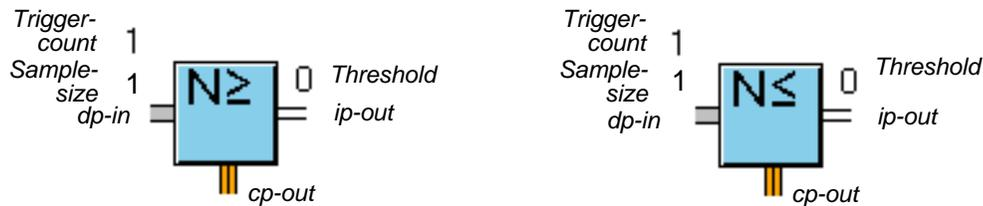
The High Pattern block and Low Pattern block test whether a certain number of values from a history of values are above or below a Threshold attribute. The number of values that must satisfy the condition is called the Trigger Count.
