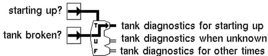
Since the top input path is `.true`, the output path labeled “T” passes the same value as the left input path. The other output paths pass unknown, the value of Status on Initialization.
