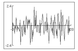
To specify the range of output values, set the attributes Disturbance Mean and Disturbance Variance. Disturbance Mean is the mean output value, and Disturbance Variance is the variance of the output values.
