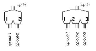
A User Query Control Switch lets you choose which control paths receive a control signal. It displays a dialog that lists radio buttons for two or three control paths, and it sends control signals down the paths you specify. The Two-Option User Query Switch lets you choose between two paths, and the Three-Option User Query Switch lets you choose between three paths.
