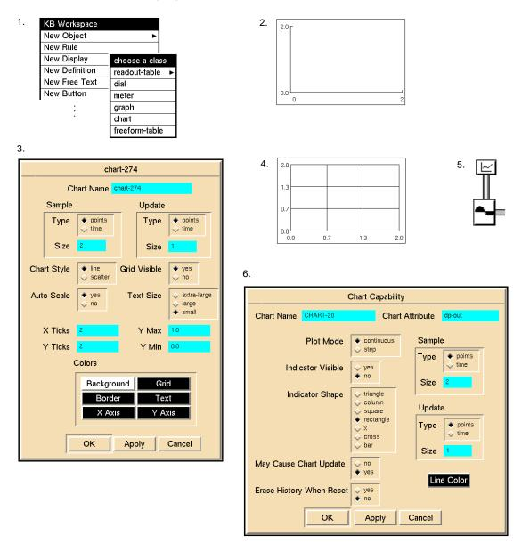
**Caution** When there is a single capability associated with a particular chart, GDA prevents you from configuring the chart and its associated capability at the same time. When there are multiple capabilities that plot data on a single chart, however, you should avoid simultaneous editing of the display and its capability, because GDA cannot prevent this.
