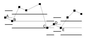
In this figure, Outlier Replacement is **yes**. Notice that when a value is out of range, the center of the new range becomes the maximum or minimum of the old
