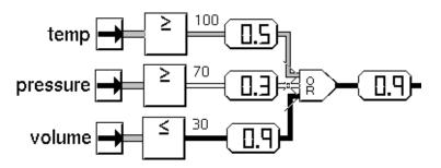
In this figure, 'D.DD' Belief Displays show you how a Weighted Evidence Combiner computes its value:
