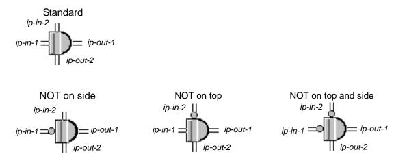
The Tabular AND Gates perform a logical AND operation. They are useful when using an AND Gate would force you to cross paths and make a diagram difficult to understand, such as when one value is an input to more than one AND Gate.
