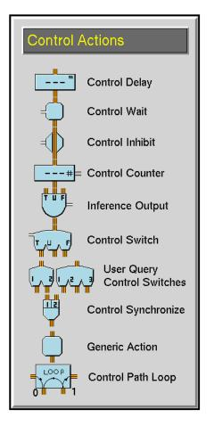
The Control Actions also let you create loops that execute actions repeatedly. To see a loop that executes a specified number of times, see the example under "Control Counter" on page 449. To see a loop that executes until some condition is met, see the example under "Control Switch" on page 454.
