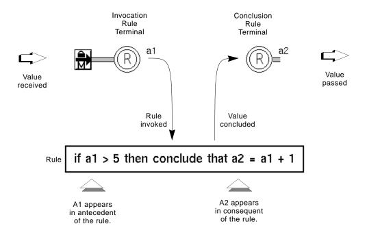
The following figure illustrates the result of passing a value of 6 into the invocation rule terminal. The figure shows the override dialog for the Numeric Entry Point and the current values of the Last Recorded Value attribute for each rule terminal.
