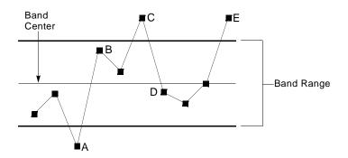
A is the first new value outside the range, so it is passed. B is the first new value to re-enter the range. C is the first new value outside the range. D is the first new value to re-enter the range again. And E is the first new value outside the range.
