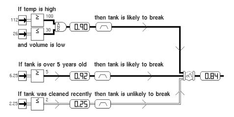
**Note** All of a Fuzzy Evidence Gate's input paths must be connected to Fuzzy Consequent blocks. It ignores the value of any input path which is not connected to a Fuzzy Consequent block.
