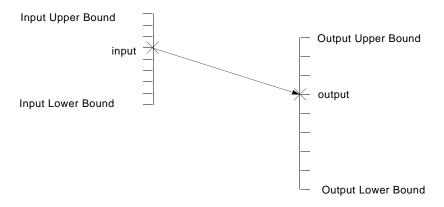
Specify the range of the input data value with the attributes Input Upper Bound and Input Lower Bound. Specify the range of the output data value with the attributes Output Upper Bound and Output Lower Bound. The block computes the output value with this equation. The variables in the equation are explained in the table that follows.
