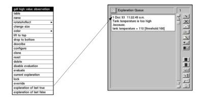
The Explanation Memory capability in this figure remembers the reason for the last alarm. The Trigger On attributes in both the Explanation Memory capability and the Alarm capability are set to .true. The Alarm Panel below the High Value block is for the alarm.
