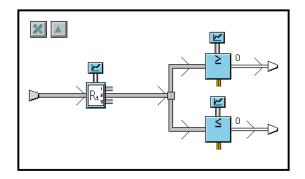
You can connect the Range Test block to Conditions, as in this figure, if you want to raise an alarm when the range falls outside the limits:
