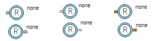
Rule terminals are G2 variables, which invoke rules and conclude values using forward chaining. Rule terminals are like any other G2 variable, in that they can keep histories and track expiration times. For a description of forward chaining and variables, see the *G2 Reference Manual*.
