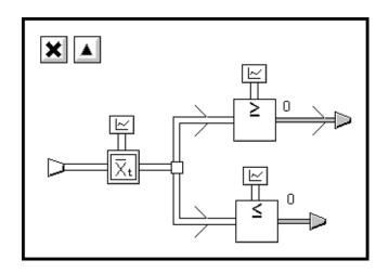
You can connect the X-Bar Test block to Conditions, as in this figure, if you want to raise an alarm when the moving average falls outside the limits:
