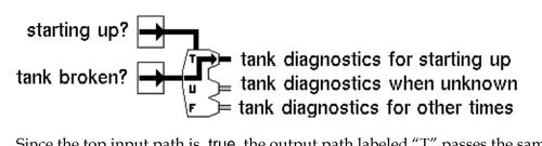
Since the top input path is .true, the output path labeled "T" passes the same value as the left input path. The other output paths pass unknown, the value of Status on Initialization.
