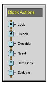
All Block Action blocks also have an Action Link, which you connect to another GDA block. When the Block Action block is evaluated, it performs its action on any block connected to its Action Link. For example, the Lock block locks any block connected to its Action Link.
