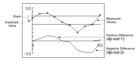
This table shows the input and output values graphed in the previous figure. Notice when the measured value moves closer to the expected value (from 2.0 to 3.5), the bottom output still decreases since the output represents a cumulative sum of the differences. Also, notice that when the measured value shoots above the expected value (to 6.25) after being below it for a long time, both output values differ from 0.
