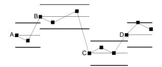
A is the original center. B is the first new value outside A's range. C is the first new value outside B's range. And D is the first new value outside C's range.
