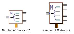
**Note** The numbering of the output ports for the Multi-state block goes from bottom to top. Thus, ip-out-1 is at the bottom of the block and ip-out-*n* is at the top. This numbering scheme corresponds to the ordering of the thresholds, which decrease as you go down the output paths.
