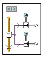
The Override Mode attribute for the Override block is set to manual by default to enable manually overriding the attached blocks.
