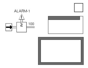
The following figure shows alarm panels for an inactive alarm that has no unacknowledged messages:
