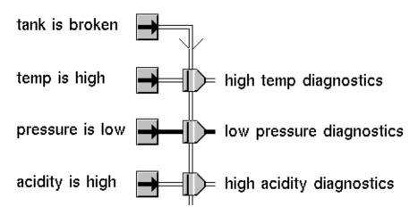
This diagram works the same as the previous diagram, even though the first Entry Point has the opposite meaning from the first entry point in the previous example. Notice that the first Tabular OR Gate has a NOT indicator on top. It inverts the Entry Point's value and passes the inverted value to the other Tabular OR Gates.
