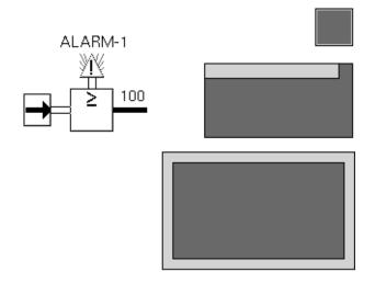
The following figure shows alarm panels for an active alarm that you have acknowledged.
