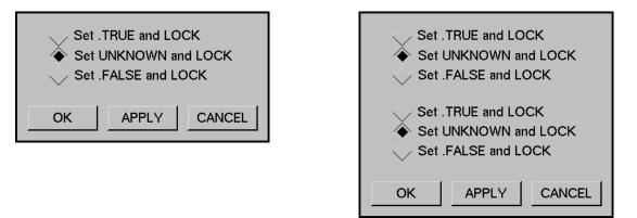
The following figure shows the default dialogs for Three-Output and Four-Output User Query blocks.
