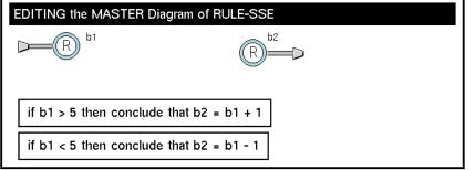
**Note** If you have created multiple instances of a Single Source Encapsulation block that contains rule terminals, GDA only invokes the rules associated with the instance that received a value; it does not invoke rules associated with every instance of the particular class of SSE block.
