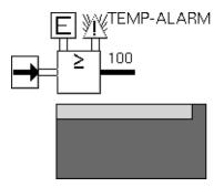
To see the saved explanation, you can select explanation of last true from the High Value block, or you can choose explain alarm in memory from the Alarm Panel's menu, as shown in this figure:
