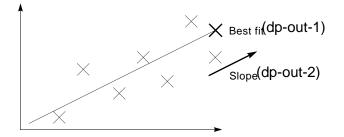
This block is frequently used with a Linear Prediction block, which predicts a future value for a point on a line. The Linear Prediction block's input values are the same as the Linear Fit block's output values (a point on a line and the line's slope) so you can connect a Linear Fit block directly to a Linear Prediction block.
