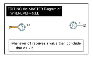
GDA also supports the and when syntax in conjunction with whenever rules. In the following example, the rule is invoked whenever c2 receives a value and when d2 is greater than 5. The rule concludes a value for d3.
