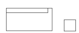
A Local Alarm Panel lets you monitor and manipulate an alarm. They come in three sizes: large, medium, and small. Color regions in the alarm panel reflect the severity of past and present alarm messages. Indicators in the alarm reflect whether there is a recurring alarm, whether the condition attached to the alarm is overridden, and more. The alarm panel's menu contains choices that let you acknowledge the alarm, view the alarm messages, override the condition, and more.
