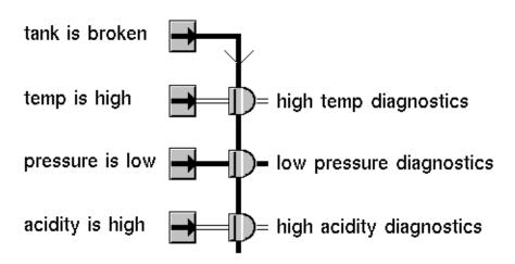
This diagram works the same the previous diagram, even though the first Entry Point has the opposite meaning from the first entry point in the previous example. Notice that the first Tabular AND Gate has a NOT indicator on top. It inverts the Entry Point's value and passes the inverted value to the other Tabular AND Gates.
