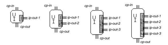
A User Query block lets you choose the output value for 1 to 4 inference paths. The block displays a dialog with three radio buttons for each path: .true, unknown, and .false. The dialog looks like several override dialogs combined together.
