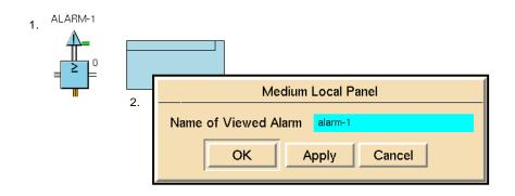
**Note** If you enter an incorrect name into the Name of Viewed Alarm attribute for a Local Alarm Panel, GDA displays an error message in the error queue and an "E" on the panel. To remove the "E" from the panel, reset the panel.
