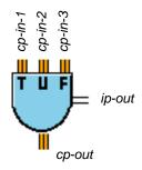
The Inference Output block chooses an inference value to pass depending on which input control path it receives a signal from. Whenever it receives a control signal on one of its input control paths, it passes the inference value for that path on its output inference path and passes the control signal on its output control path.
