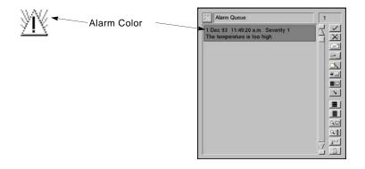
These are the default colors for the severity levels: 1 is red, 2 is orange, 3 is gold, and the rest are gray. You can change the colors with the Alarm Colors palette. To use the Alarm Colors palette, bring up the Configuration Tools menu bar, go to the Colors menu, and choose Alarm Colors.
