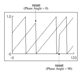
If you change Phase Angle as GDA is running, GDA uses the new value the next time you reset the block.
