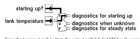
Since the top input path is .true, the output path labeled "T" has the same value as the left input path. The other output paths are none, the value of Value on Initialization.
