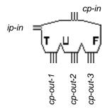
The Control Switch lets an inference value choose which path to send a control signal down. It is useful when you need to perform a sequence of control blocks until some condition is met.
