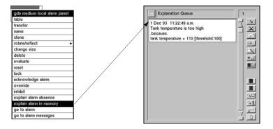
If you have more than one Explanation Memory capability attached to a block, the explain alarm in memory menu choice displays only the latest explanation created.
