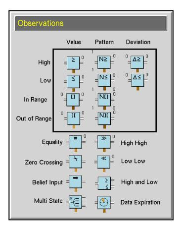
All observations have similar icons. A symbol on the block indicates the test the block performs. This figure shows the High Value Observation. The symbol " $\geq$ " means the block performs the test greater-than-or-equal-to.
