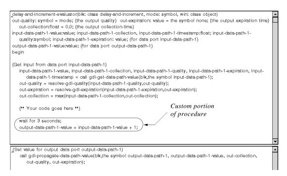
The following table shows sample input and output values for this block. The input and output values update once a second. The output values increment the input value associated with  $t_{n-3}$  by 1.
